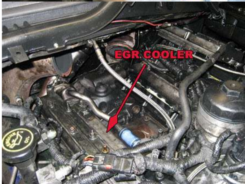
EGR cooler can suffer coolant starvation, overheat and crack Credit: PowerStorke.org
