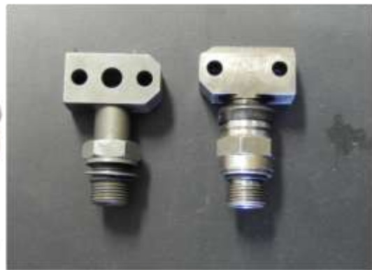
STC connector: New style (L), Old style -(R) Credit: Bulletproof Diesel
