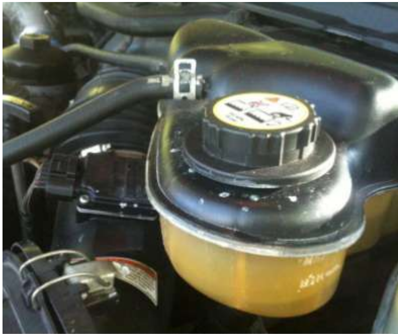
Coolant degas bottle often suffers from broken drain neck and leaking cap.
