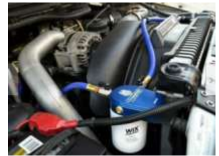
5 Coolant Bypass Filter
