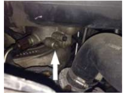
8 Fuel Pressure Test Port
